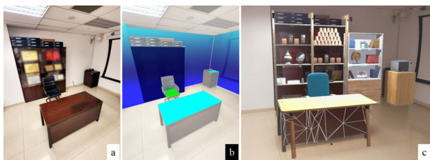
Fig. 3 a The original real scene. b The interactive surfaces where vertical haptic planes are highlighted in blue and horizontal haptic planes are highlighted in cyan or green. c Dual-pass mixed scene rendering by HoloLens 2 with disocclusion
